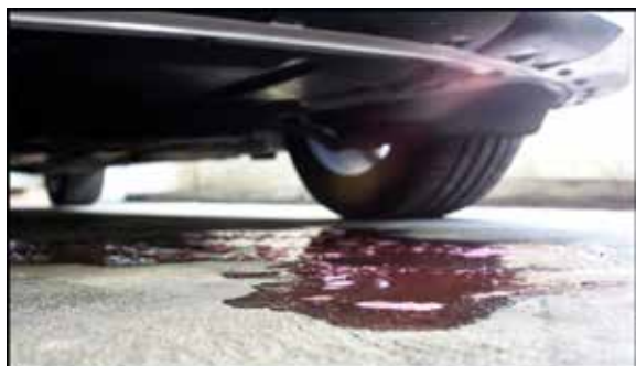
Antifreeze leaking from a car.
